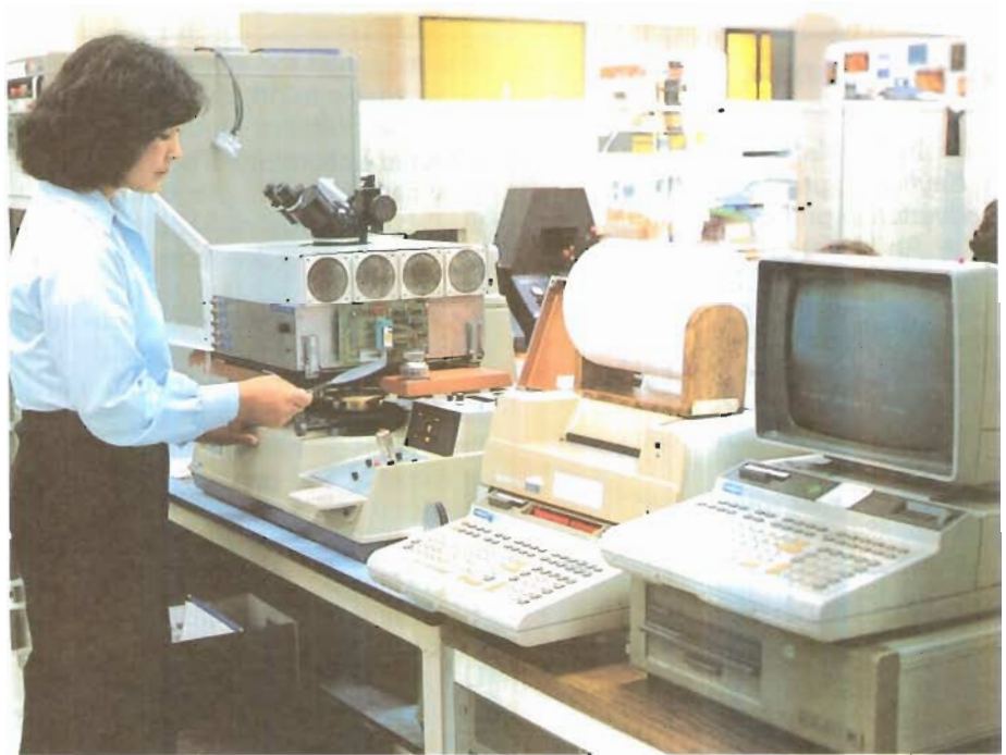
HP employee Koko Jacobs unloads a 100 mm wafer from the prober. The defective ROMs have been inked and the failure locations sent to the HP 9825.
