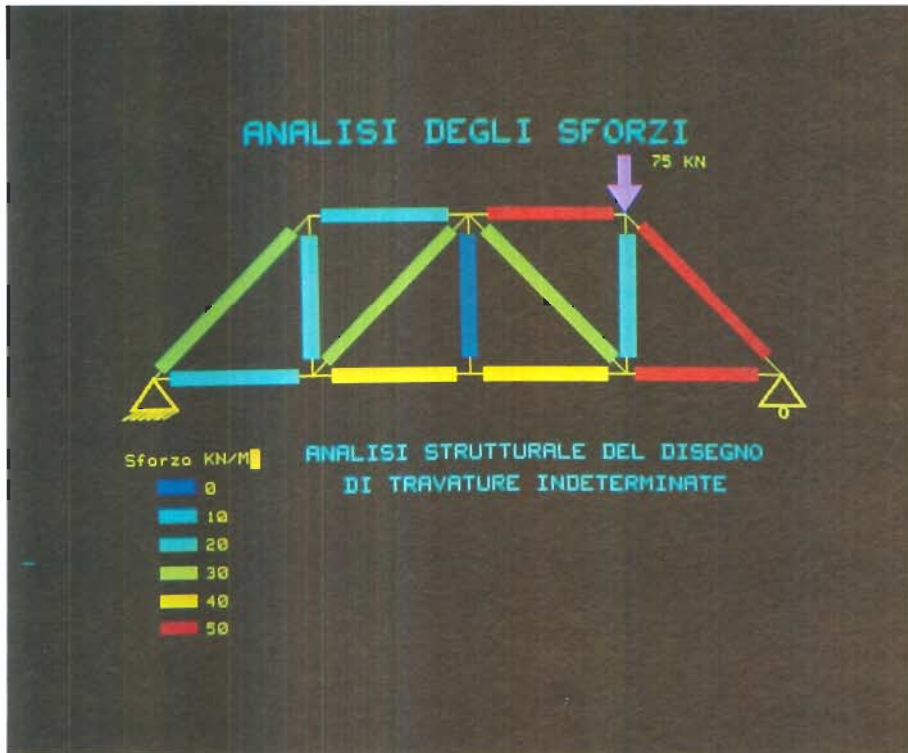
Stresses on a bridge design are shown in colors that denote the degree of stress in this image generated on the System 45C. Labels in this image are presented in Italian.
